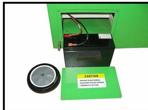
cage, you will find 2 wires which should be connected to the battery terminals. The red wire should be connected to the red terminal and black wire to the black terminal. Care must be taken to ensure you put the battery terminals to the top left side when you insert the battery into the cage
