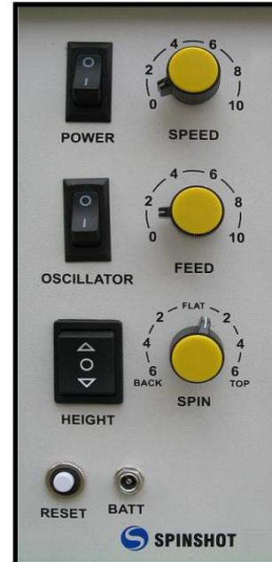
**HEIGHT:** Pushing 'HEIGHT' upward will raise the ball trajectory, and pushing downward lowers the trajectory. The elevation control automatically stops at both the highest and lowest possible trajectories.
